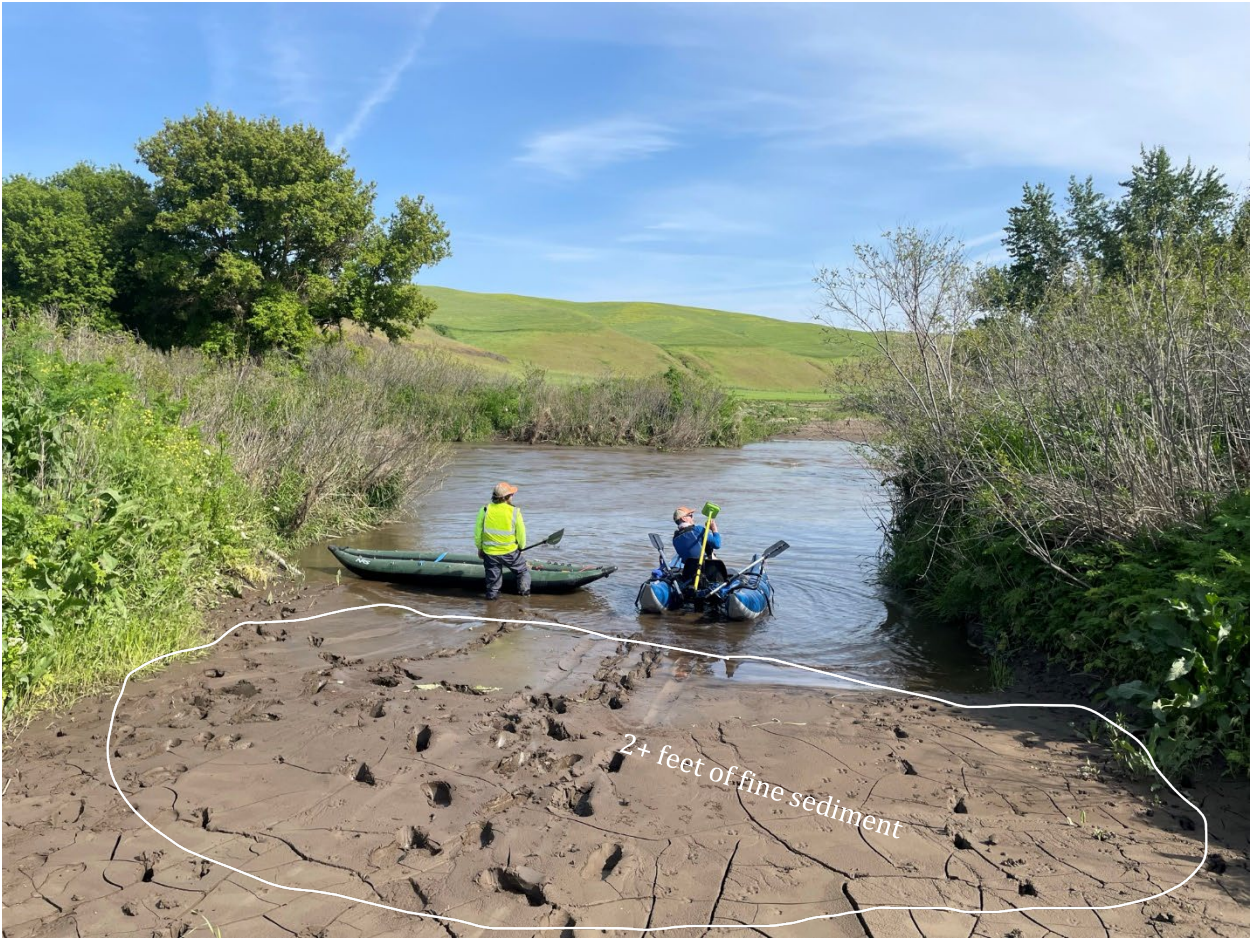
Figure 31: Fine sediment along the banks near RM 15.7. Deposit was from a single year of spring runoff flows.
