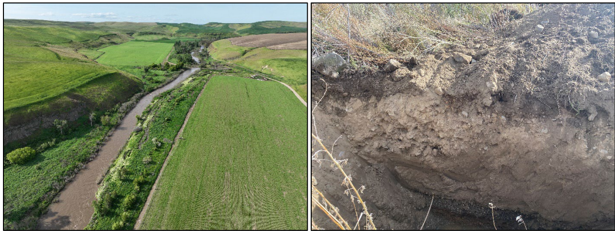
Figure 9: Photo of straightened channel segment at the project site (left). Photo of test pit excavated along the right bank of the photo at left showing substantial coarse, angular non-alluvial material likely placed during the channelization process.
